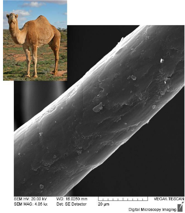
Fig. 5 Picture of Camel fibres taken by SEM microscopy (animal picture [21])
