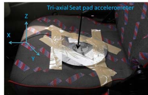
Fig. 3 Measurement location on Seat pad accelerometer
