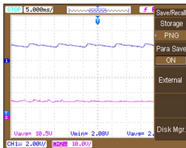
Fig. 7 Measurement waveform first stage output with 10x attenuation (upper) and dc-dc output (lower)
