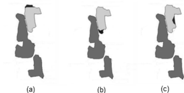
Fig. 14: Location of the silt (in dark) input point considered for the modeling: (a) upstream, (b) downstream and (c) laterally the quarry lake, with reference to the groundwater flow direction. In light gray is shown the active quarry lake with the dimensions provided for its expansion, whereas in deeper gray are shown the quarry lakes not directly interested by the intervention
