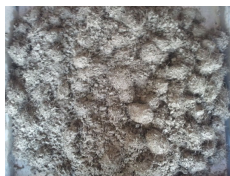
Fig. 4 Fiber ball Phenomenon (S44F1.25, S44V1.5, S51V1.5)
