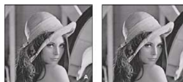
Fig. 18. A) Cover Image B) Stego Image of Lena after embedding "I am an Indian and I feel proud to an Indian."
