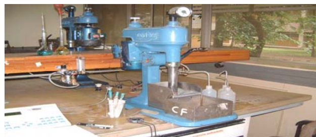
Fig. 4 Laboratory flotation machine, Denver D 12
