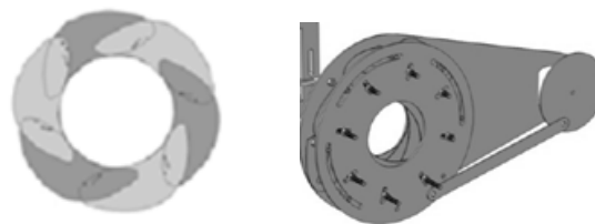
Fig. 3 Our most recent variable aperture design [6]
