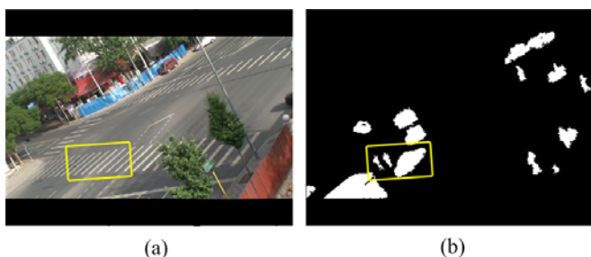
Fig. 8 Pedestrian-vehicle traffic conflict detected by improved algorithm: (a) subtracted background; and (b) extracted moving objects
