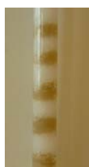
Fig. 2 Column reactor filled with sol-gel immobilized Alcalase and ammonium carbamate
