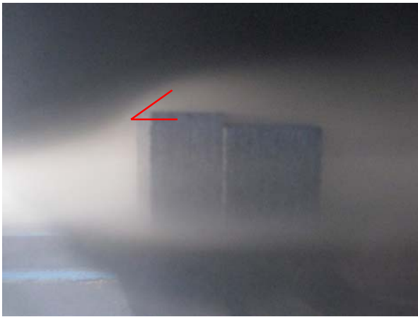
Fig. 9 Main flow features on the vertical plane passing from the WECS mounting point and oriented from NE to SW; the inclination of the separation bubble at the leading edge of the roof is evidenced by the red lines
