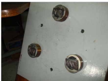
Fig. 2 The arrangement of the specimen holders and test pieces attached underneath the sled
