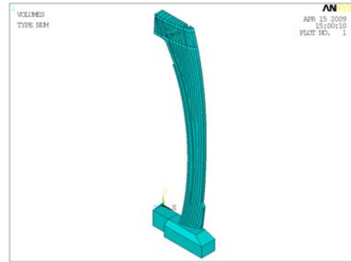
Fig. 3 Finite element mesh of the cable tower
