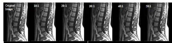
Fig. 2 Comparison between original and compressed MRI Spine images
