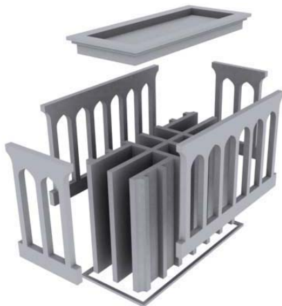
Fig. 6. 3D model of a Wind catcher with different canals
