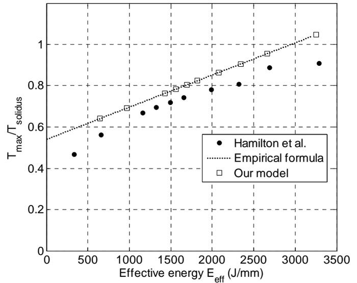
Fig. 6 Variation of the maximum temperature with the energy level for our model, Hamilton's model, and the experimental results.
