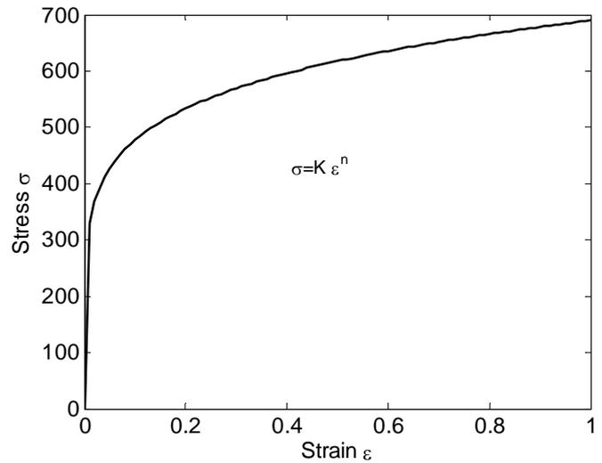
Fig. 3 True-stress true-strain curve for AA 2024.
