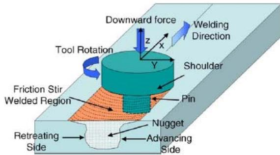
Fig. 1 A schematic of friction-stir welding process.
