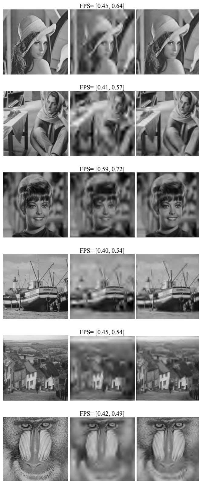
Fig. 10 Foveation Probability Score FPS Evaluation for Lena, Barbara, Zelda, Boat, Goldhill and Mandrill test images for a viewing distance of V = 4 . The FPS factors quality are given for each test image (left column: original images) coded at a bit rate of 0.03125 bpp (middle column: low bit rate) and 0.125 bpp (right column: high bit rate)
