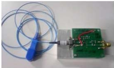
Fig.2 Configuration of ROSA PIN-PD with Pre-Amplifier
