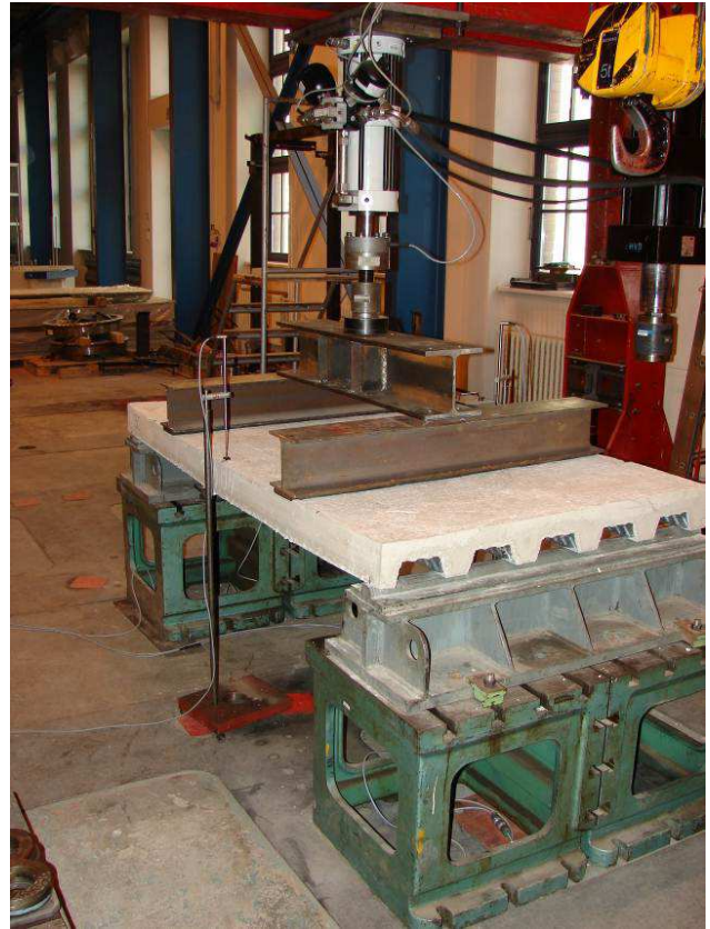
Fig. 7 Four-point bending. Configuration of the test setup
