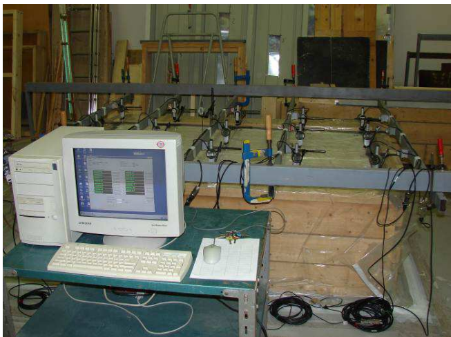
Fig. 6 Vacuum loading. Configuration of the measuring devices for monitoring slab deflection
