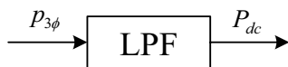
Fig. 3 The separation of the fundamental power from the three-phase power using LPF
