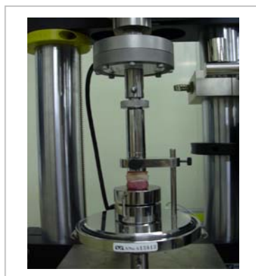
Fig. 4 Configuration of the compressive test using Instron Microtest System (5848 series, Instron, Norwood, MA, USA)
