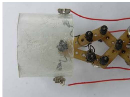
Fig. 8 The turning mechanism of the robot
