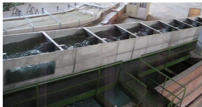
Fig. 1. Fishway model used in experiments.
