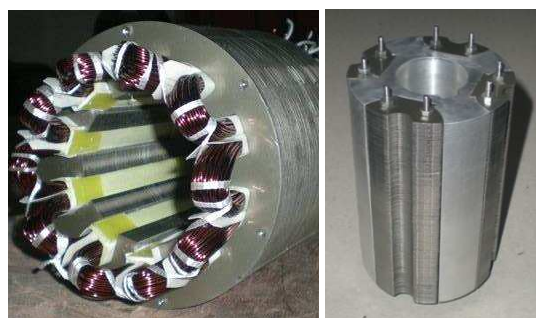
(a) Front views of the stator and rotor before they are joined to other parts and placed into frame
