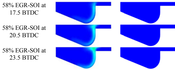
Fig. 16b Contour plots of soot (left) and NOx (right) mass fraction at different SOI at 360 °C
