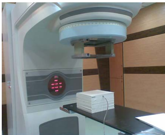
Fig. 2 set up for parallel-plate chamber measurements
