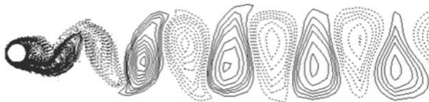
Fig.5 vortex mode in the wake of flow past a fixed cylinder
