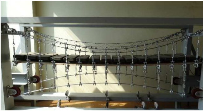
Fig. 12 Model of cable truss top chord
