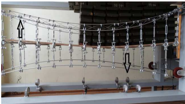
Fig. 23 Displacements in non-symmetrical loading case
