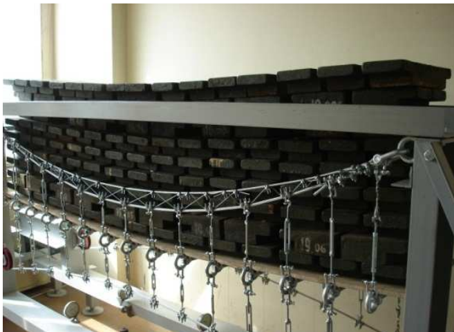
Fig. 21 Applying symmetrical load to the model
