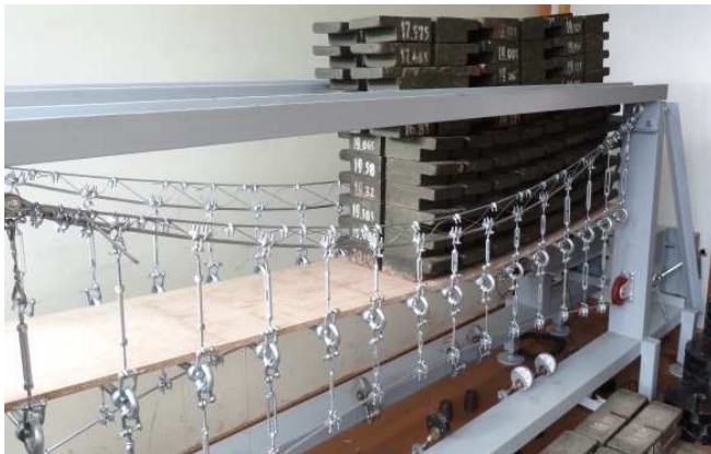
Fig. 22 Applying non-symmetrical load to the model
