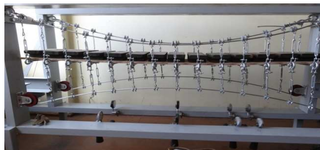
Fig. 11 Model of single cable top chord
