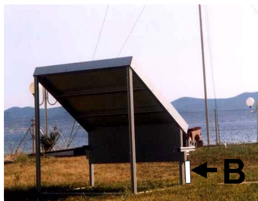
Fig. 1. The dew condenser (1m x 1m surface area) at the Zadar station (Croatia). Collection is made in a PE bottle (B)
