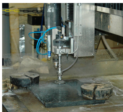
Fig. 4 Cutting of a test sample from a 30mm thick plaque using a water-jet cutter
