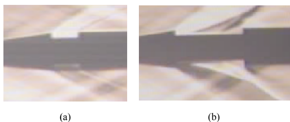
Fig. 3 Schlieren images for open-cavity of L/D=4 (3a) and closed-cavity of L/D=12 (3b) on the right
