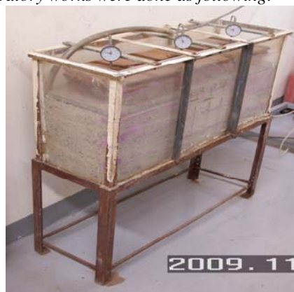
Fig. 1 Model shape with volume change measuring unites
