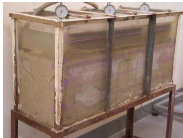
Fig. 7 Picture of sub surface submerging
