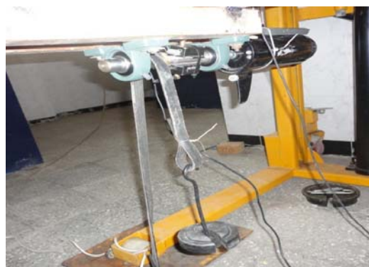
Fig. 5 Propeller torque measurement test rig
