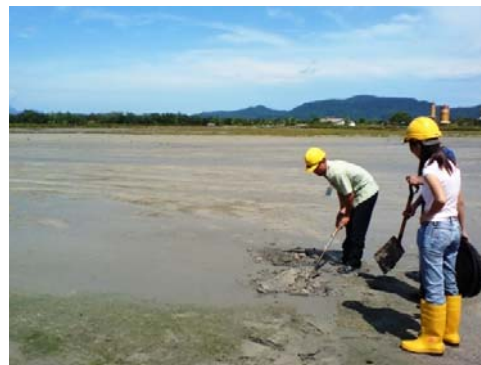
Fig. 3 PA sample collection at ash disposal site, Sejingkat Thermal Power Plant, Kuching
