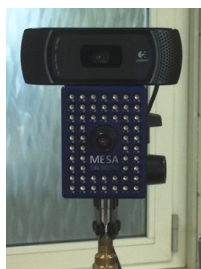
Fig. 1. The two cameras used in the experiments: the SR3000 (bottom) and the Logitech HD Pro Webcam C910 (top)
