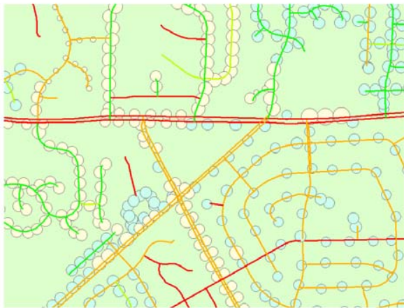
Fig. 3 Intersection between the effectively lit circle with the centerline of streets. Blue circles represent Mercury Vapor lamps. Two lines represent centerline of two way streets.
