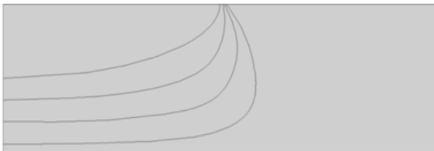
Fig. 15 The crack shape development for a deep semi-elliptical surface crack a/c=0.33 , a/w=0.5 under ductile tearing in tension
