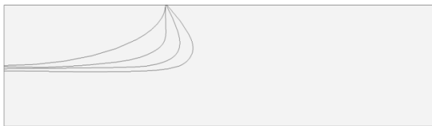
Fig. 10 Crack shape sequence for a deep semi-elliptical surface crack under bending ( a/w=0.5 , a/c=0.33 )
