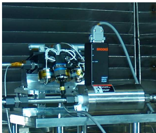
Fig. 3 Thruster on the thrust stand
