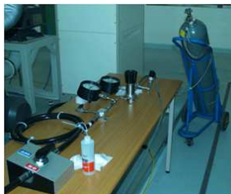
Fig. 7 High pressure nitrogen tank and propellant supply line
