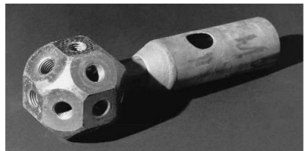
Fig. 4 1-Standard MERO KK node with 18 threaded holes and machined bearing surfaces at angles of 45°, 60° and 90°
