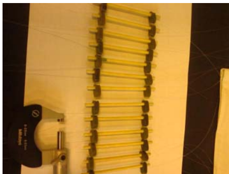
Fig. 3. As-prepared wound mandrels for aging treatment
