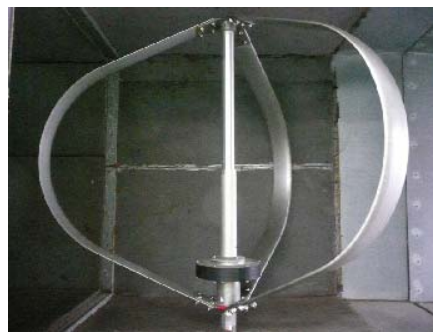
Fig. 2 Darrieus type VAWT for wind tunnel experiments
