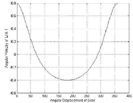
Fig.5: Angular velocity of link 1 ( $\omega_2$ )
