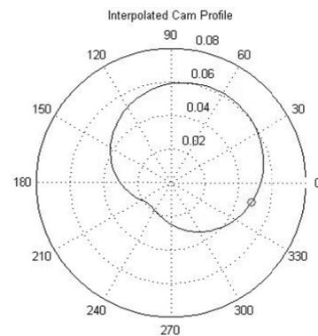
Fig. 9: Interpolated cam profile
