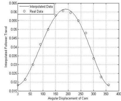
Fig. 8: Interpolated follower displacement and real data
