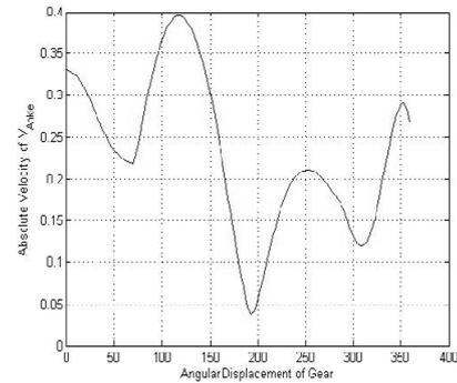
Fig. 15: Definitive absolute velocity of  $V_{Ankle}$  for one cycle
