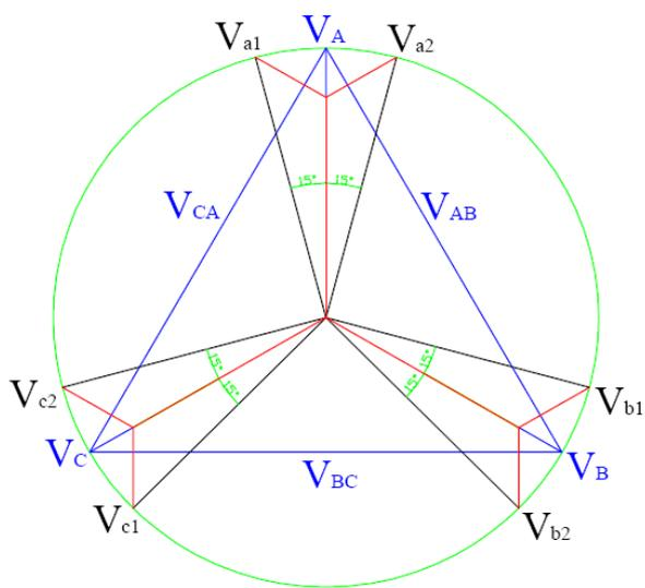
Fig. 2 star connection of proposed autotransformer for 12-pulse converter and its phasor representation
