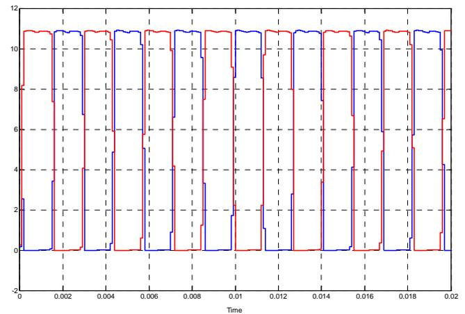
Fig. 11 Diodes  $D_1$  and  $D_2$  current waveforms
