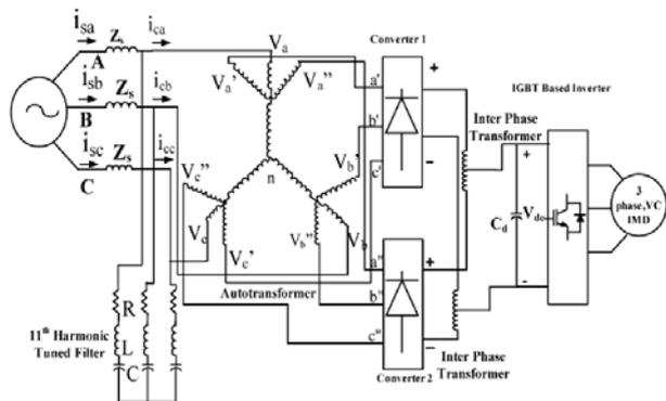
Fig. 1 star-connected autotransformer configuration for 12-pulse ac-dc conversion [12]
