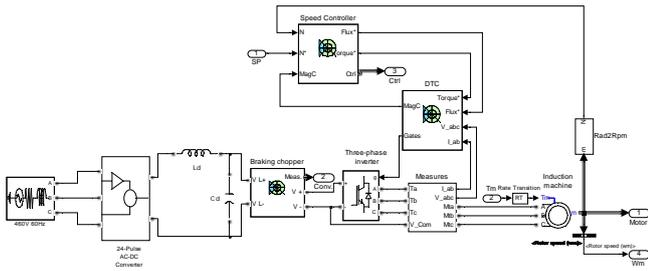
Fig. 6 Matlab model of 24-pulse ac-dc converter fed DTCIMD
