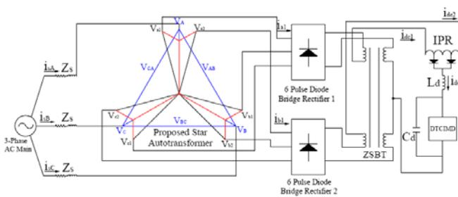
Fig. 3 star-connected autotransformer configuration for 24-pulse ac-dc conversion
