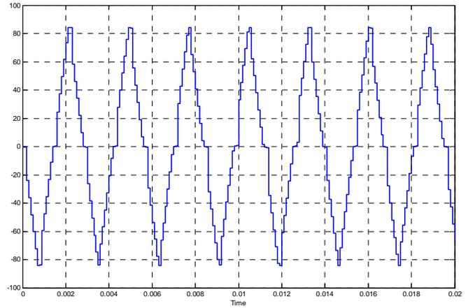
Fig. 10 Voltage waveform across the double-tap IPT
