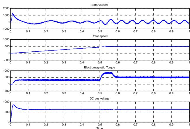
Fig. 13 Waveforms depicting dynamic response of 24-pulse diode rectifier fed DTCIMD with load perturbation (source current  $i_{SA}$ , speed  $\omega_r$ , developed electromagnetic torque  $T_e$ , and dc-link voltage  $V_{dc}$ )
