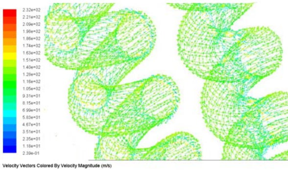
Fig. 11 Velocity vectors for cooling ducts having turbulators of e/D = 0.04 and 0.75mm rib thickness
