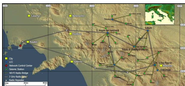
Fig. 3 Topology of communication system of Irpinia Seismic Network (ISNet) in southern Italy
