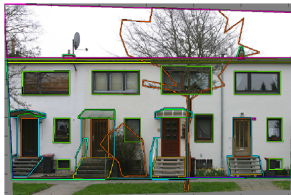
Fig. 1. Example from the eTRIMS annotated façade database. Each object is marked by a bounding polygon and a label from the ontology (indicated here by different colours.)
