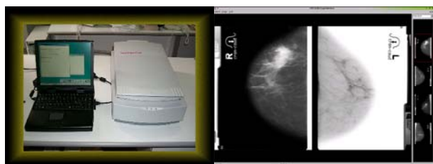
Fig. 1 A portable CAD unit of the MAGIC-5 project and the graphical users interface
