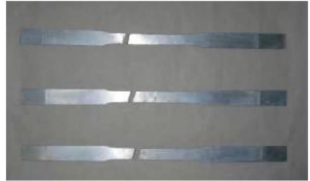
Fig. 4 The samples after tensile test experimental test
