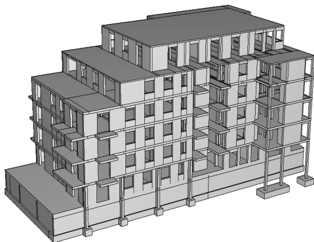
Fig. 3 Finite element model of the multi-storey RC building
