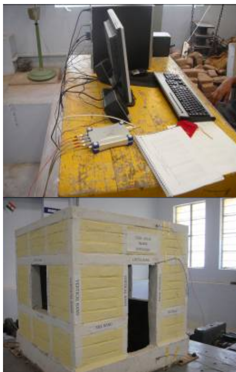
Fig. 9 Instrumentation and location of Accelerometers
